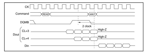
**2. Same bank, different ROW address:** When the ROW address changes, consecutive write commands cannot be executed; it is necessary to separate the two commands with a precharge command and a bank-active command.
