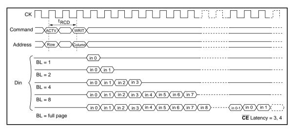
**2. Single write:** A single write operation is enabled by setting OPCODE (A9, A8) to (1, 0). In a single write operation, data is only written to the column address and the bank select address (BA) specified by the write command set cycle without regard to the burst length setting. (The latency of data input is 1 clock).
