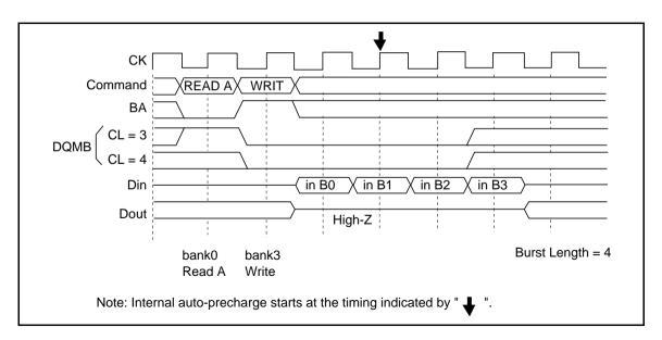
**2.** Same bank: The consecutive write command from read with auto precharge (the same bank) is illegal. It is necessary to separate the two commands with a bank active command.
