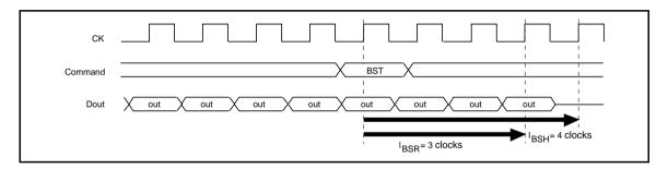
**Burst stop command at burst write:** The burst stop command (BST command) is used to stop data input during a full-page burst write. No data is written in the same clock as the BST command, and in subsequent clocks. In addition, the BST command is only valid during full-page burst mode, and is illegal with burst lengths of 1, 2, 4 and 8. And an interval of  $t_{DPL}$  is required between last data-in and the next precharge command.
